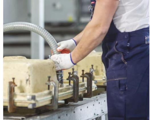
The Laveo granite sinks are manufactured in the 80:20 ratio from a mixture of granite, responsible for product durability, and polyester resin.
