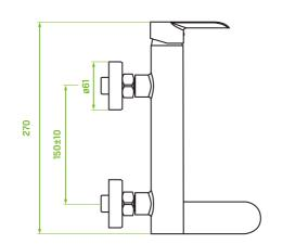
Alea 3-hole bath mixer is designed for upright installation directly on a bathtub or in a shelf covered with tiles. Shower hose is concealed under tiles or bathtub.
