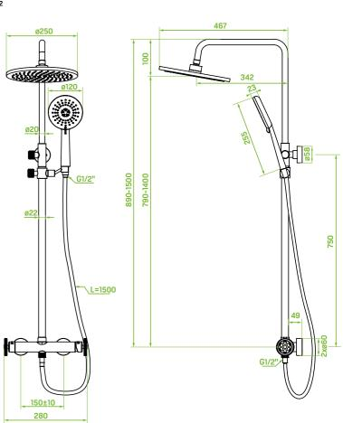
Shower column fitted with a mixer with special thermostatic cartridge allows to set a desired water temperature, the same any time the **Kvadrato series**allows to set a desired water temperature, the same any time the stream is activated. It gives a possibility to set a desired constant water temperature, without a risk of burns. This solution is popular in flats occupied by elderly people and families with small children for safety
