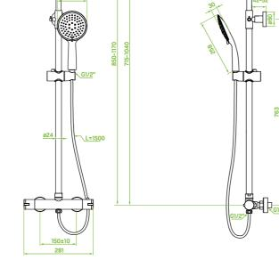
Shower column fitted with a mixer with special thermostatic cartridge allows to set a desired water temperature, the same any time the
