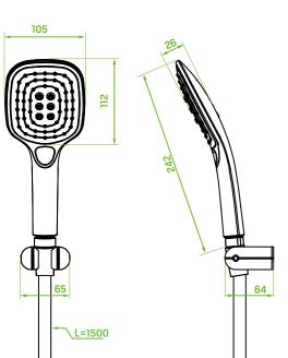
Water stream is changed with a button located in hand
